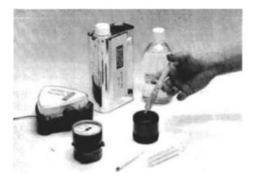
3. Shake the bottle with TBN Solution and fill a new and clean syringe with 10 ml of TBN Solution. Place the syringe in the opening of the notched lid and empty the syringe.
