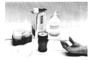
Remove the syringe and immediately close the valve by turning the notched lid to 'S' (clockwise) making sure the pressure is zero when starting the reaction.
