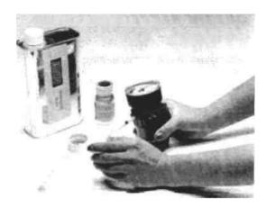
5. Remove the syringe and immediately close the valve by turning the notched wheel to 'S' (clockwise) assuring the pressure is zero.
