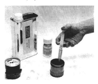
2. Add 5 ml water-free diluent using a new and clean 5 ml syringe.
